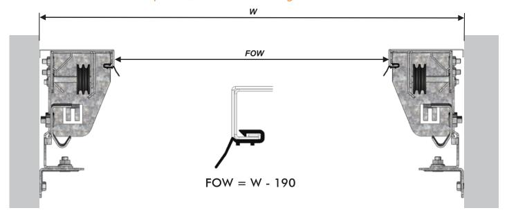
2. Optional – vertical cover profile "L" with low sealing. Installation to match the facade of the house.
