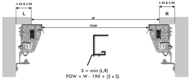
3. Optional – at side room ≥ 1 and < 24 mm, vertical cover profile "J" with low sealing; painting to RAL/NSC on request
