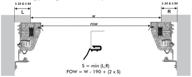
2. Optional – at side room  $\geq$  24 and  $\leq$  94 mm, vertical sealing with broken thermal bridge
